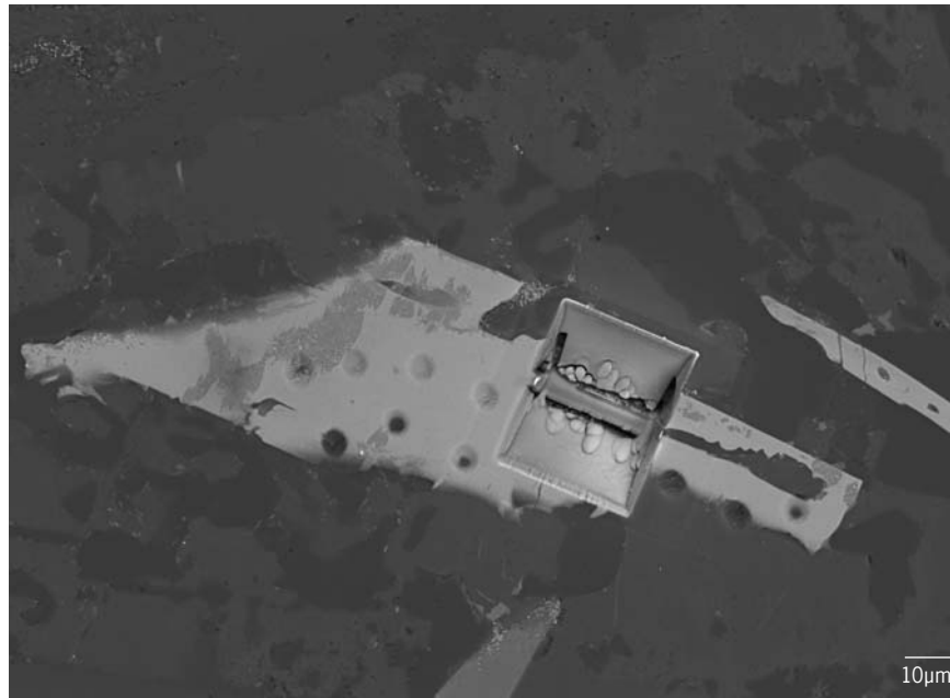
Scanning electron micrograph of a grain of tranquillityite after SHRIMP analysis and removal of a FIB section.
