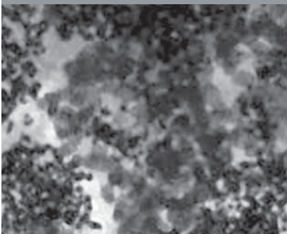
TEM image of the 100 nanometre diameter gold-coated magnetic nanoparticles.
