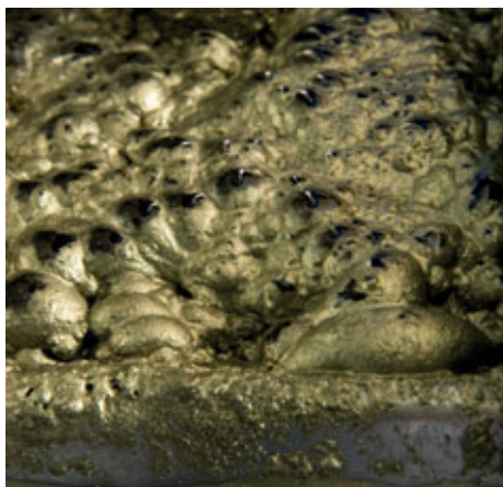
Froth flotation of chalcopyrite, a copper-iron-sulfide mineral. Photograph courtesy of Sam Noonan.
