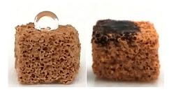
The polymer sponge absorbs oil while resisting seawater. This makes it ideal for cleaning up water based contaminants.
