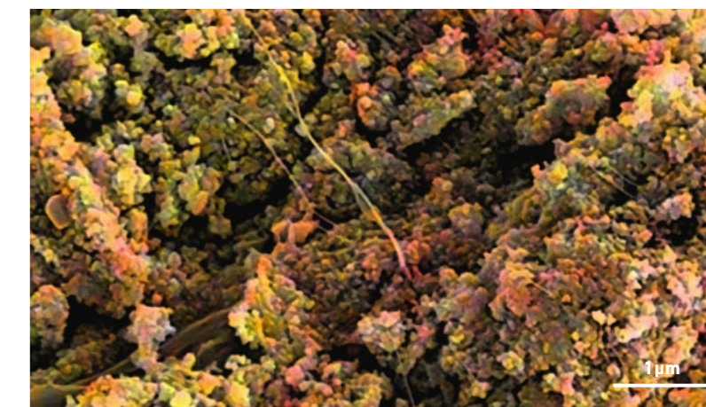
Scanning electron microscope images, overlaid with an elemental map showing the structural differences in electrodes with (bottom) and without (top) glucose. Without glucose the binding material (red) covers the sulfur (yellow), whereas with glucose, the structure is more open and more sulfur is exposed so it can interact with lithium.
